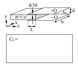
c) What is the magnitude and direction of the force  $\overline{f}$  on the new plate of Part (b) as a function of the insertion distance L. Please express your answer as a function of the parameters given in the figure.
