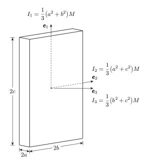
Figure 3: Local coordinate frame and moments of inertia for a parallelepiped book.
