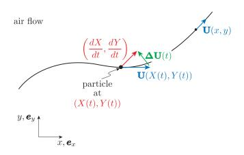
Figure 2: A particle at position (X(t), Y(t)) in an air flowfield  $\mathbf{U}(x, y)$ .
