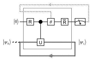
Note that an additional component is added in the control path, a  $\theta$  box, which implements the transform
