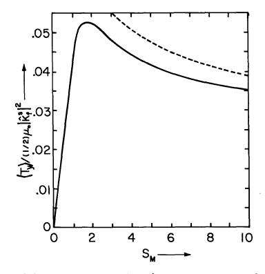
Fig. 6.6.2. Time-average force/unit area acting on deep conductor in direction of traveling wave. ka=kd=1,  $\mu=\mu_0$ . The force is an odd function of  $S_M \equiv \mu\sigma a^2(\omega - kU)$ . The broken curve is the high-frequency asymptote given by Eq. 11.
