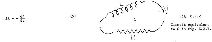
In the limit of "infinite" conductivity, the flux intercepted by a surface of fixed identity is invariant Equations 3 and 4 represent the same laws, so if the left side of Eq. 3 is negligible, it too implies that the flux linking a contour of fixed identity is conserved. The circuit helps to emphasize that in most of the chapter the subject is distributed "resistors" and "inductors" typified in their dynamics by "L/R" time constants.
