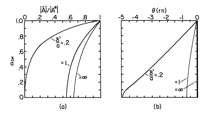
Fig. 6.6.3. Amplitude and phase of  $A = \operatorname{Re}|\hat{A}(x)|\exp j(\omega t - ky + \theta(x))|$  for fields diffusing through conductors of Fig. 6.6.1. The parameter is the skin depth, based on the material frame frequency, normalized to the conductor thickness,  $\delta'/a$ ; ka = 1.
