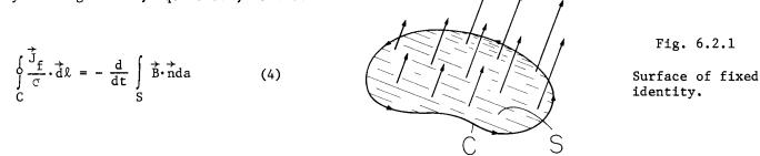
In writing this equation, the surface S enclosed by the contour C, Fig. 6.2.1, is one of fixed identity (one attached to the deforming material), so  $\vec{v} = \vec{v}_s$ . (The same expression would be obtained by integrating Eq. 3 over a surface of fixed identity and applying the generalized Leibnitz rule, Eq. 2.6.4.)
