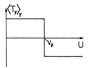
Fig. 6.11.4. Dependence of magnetic surface force density on speed for a hysteresis-type device.
