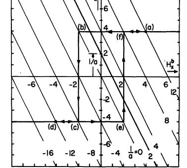
Fig. 6.11.2. Idealization of magnetization characteristic showing graphical solution (a + b)/a = 2.
